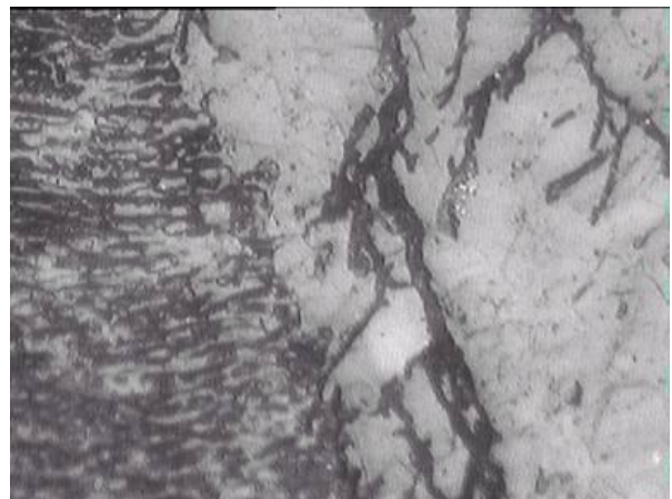
Figure 6 – Replicated Microstructure of 304 SS Reactor Showing Trans Granular Stress Corrosion Damage at HAZ (400X)
